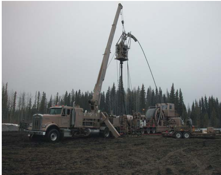
Figure 4 Typical Horseshoe Canyon nitrogen completion using coiled tubing (Source: CSUG)
